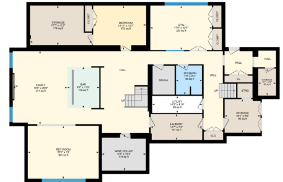
Basement (Below Grade) Finished Area 2993.54 sq ft Unfinished Area 68.77 sq ft
